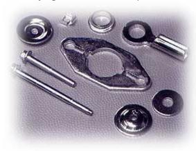
requires no additional steps or secondary top coats. Under mild agitation (either mechanical or solution circulation) and an immersion time of between 30 and 60 seconds, Aldokote ZNT-150 can provide a protection of more than 120 hours of neutral salt spray testing against the appearance of white corrosion, easily surpassing typical automotive and other industry specifications.
